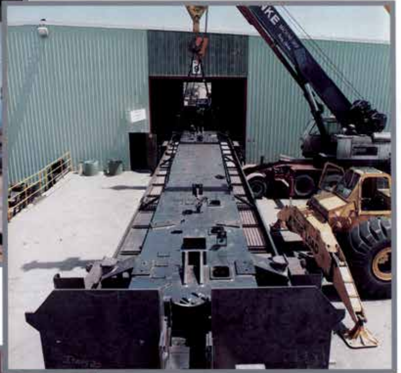
Fabrication and loadout of a 60,000 lb. train engine frame.
