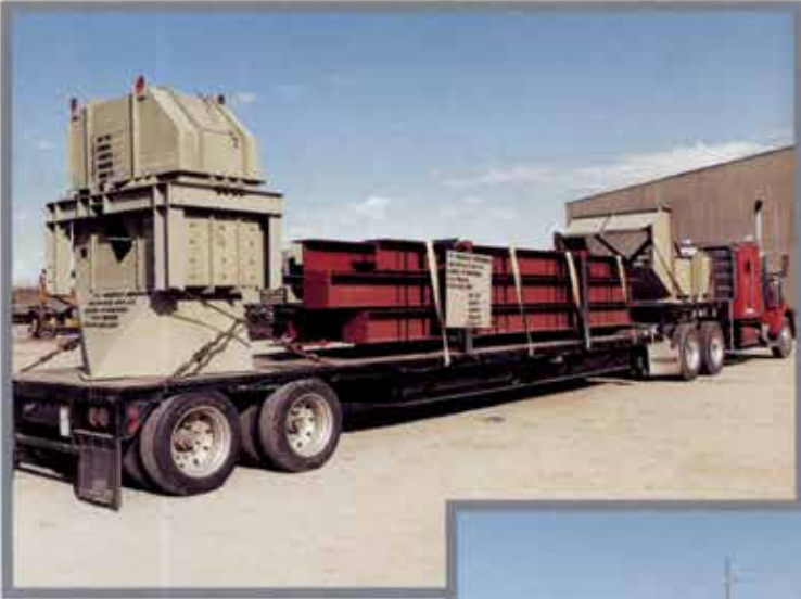
Conveyor head chutes and structural steel being transported to a port for overseas shipment to Freeport, Indonesia.
