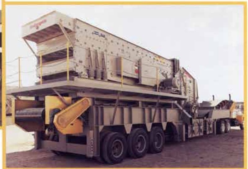
▲ Screening and crushing trailer built for a local contractor.
