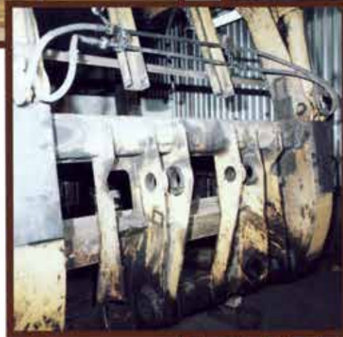
Repair and add reinforcing plates to a set of log forks. ▲
