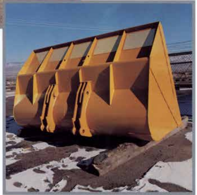
Eight yard bucket for a Caterpillar 988 loader.
