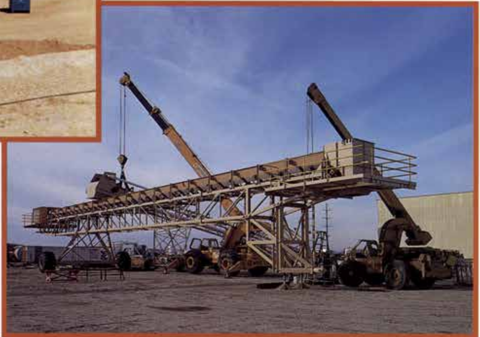
▲ Grasshopper conveyor feeding an indexing conveyor for a mine in Central Idaho.
