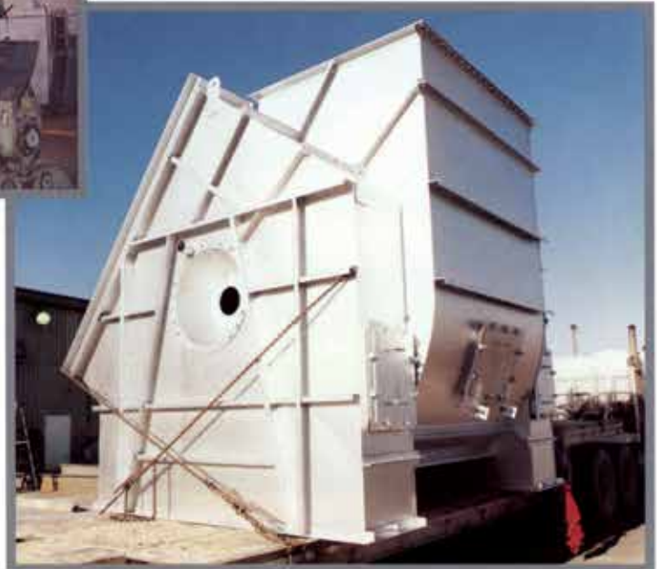
Fan housing for an air handling system at a local processing plant.
