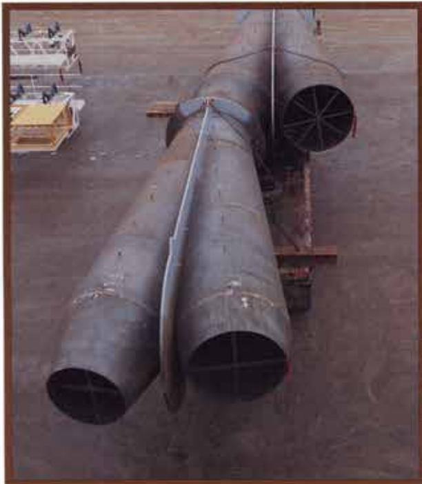
Large 7' 0" dia. water manifold split and reduced to 3' 6" dia. and 6' 6" dia. outlets. Manifold was built for a hydroelectric project in Southern Idaho.
