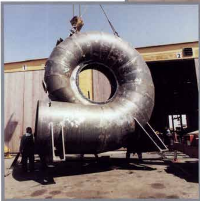
Spiral case for a hydroelectric project in Utah.
