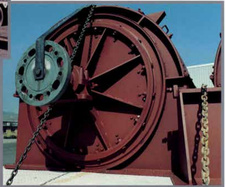
▼ Beet slicer fabricated, machined and assembled for a sugar beet processor.
