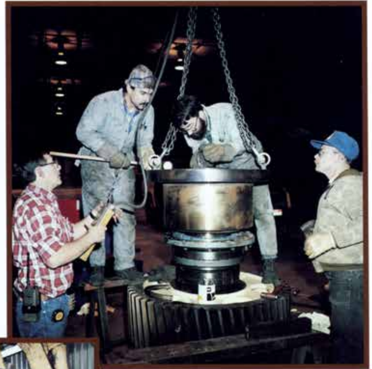
Installation of a coupling on a shaft in the Repair Shop. ▲
