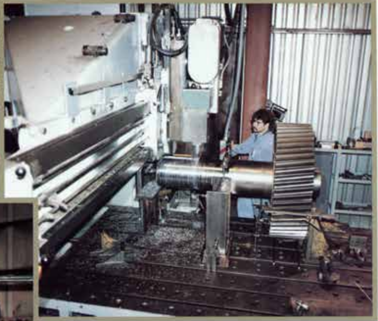
▶ Cutting a keyway on a large gearbox shaft.
