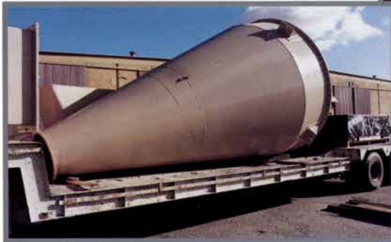
▲ Bottom conical portion of a large abrasion resistant cyclone for a plant in Eastern Oregon.
