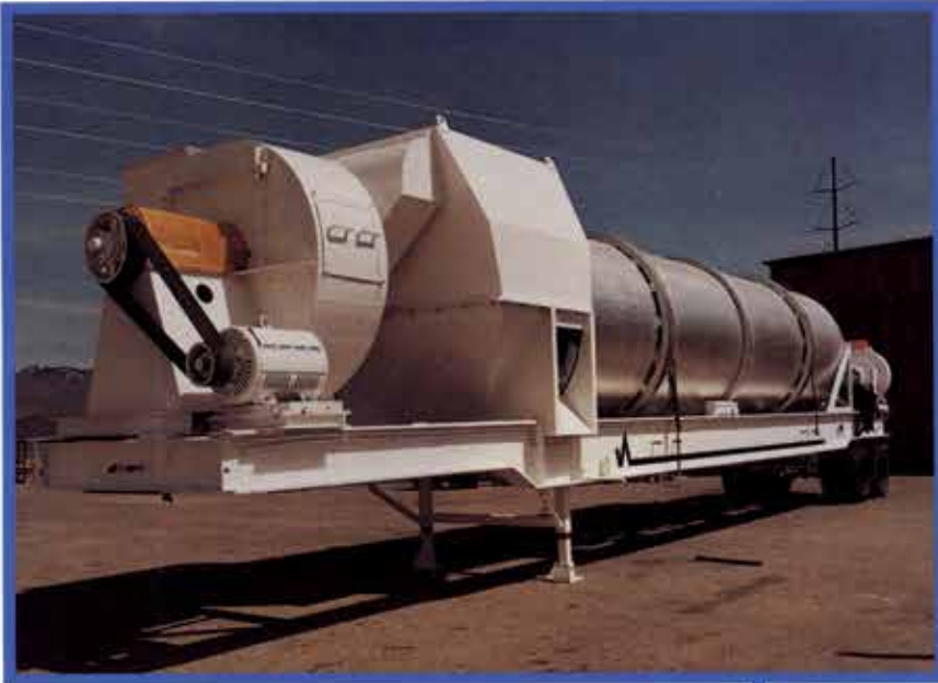
▲ 300 ton per hour asphalt drum mixer.
