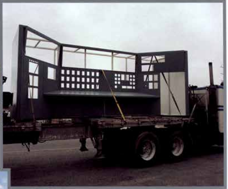
▼ Light metal fabrication of a control panel used in a wood products plant in California.
