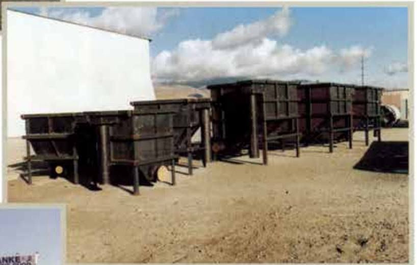
Pump boxes for a Northern Nevada mining operation. ▲
