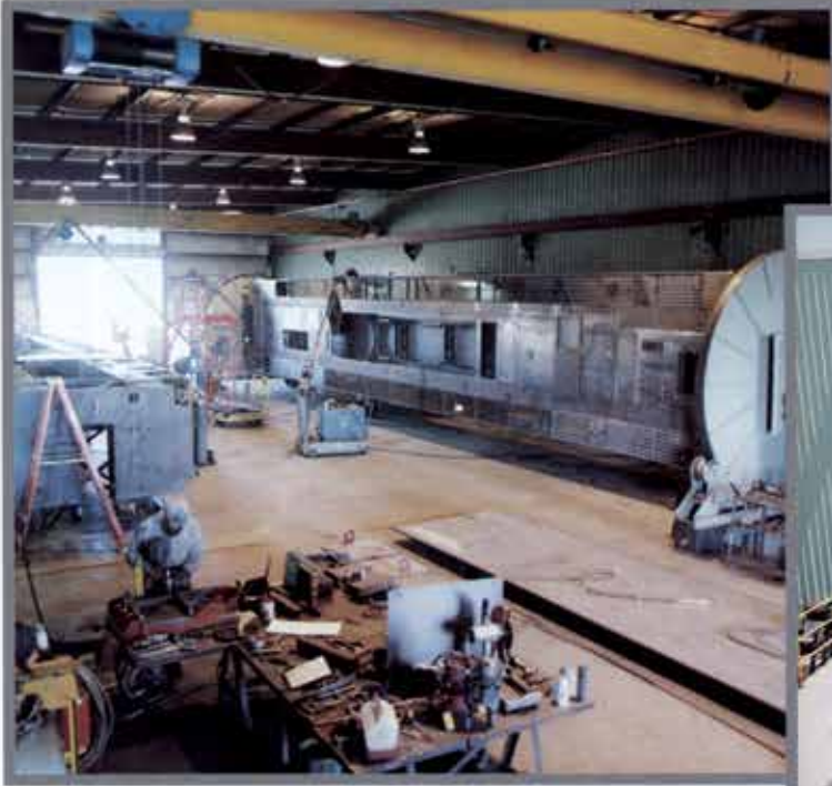
Fabrication and loadout of a 60,000 lb. train engine frame.
