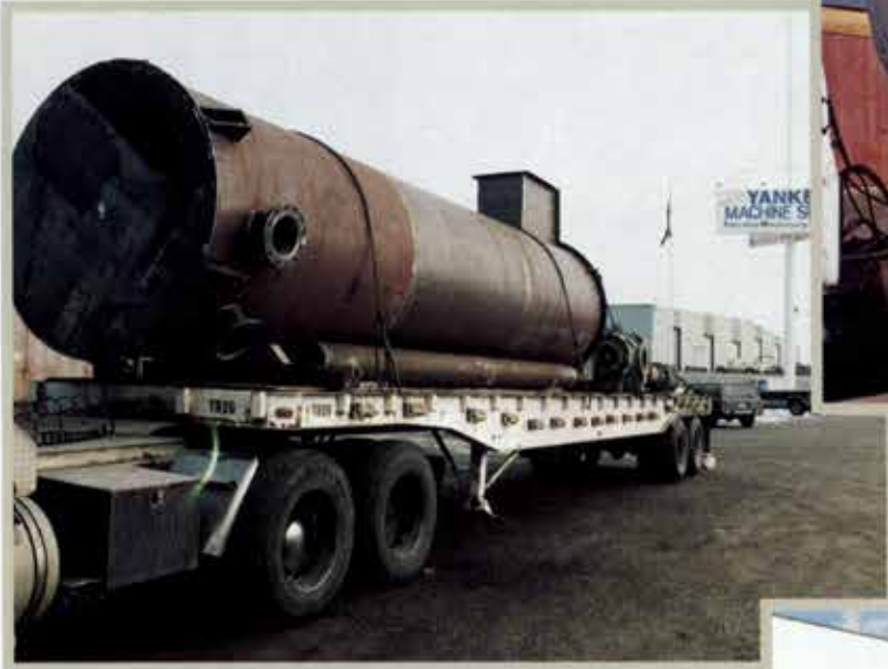
Rubber lined solution tank for a mining operation. ▲
