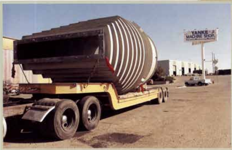
▶ Reactivated carbon storage hopper for a Nevada mine.
