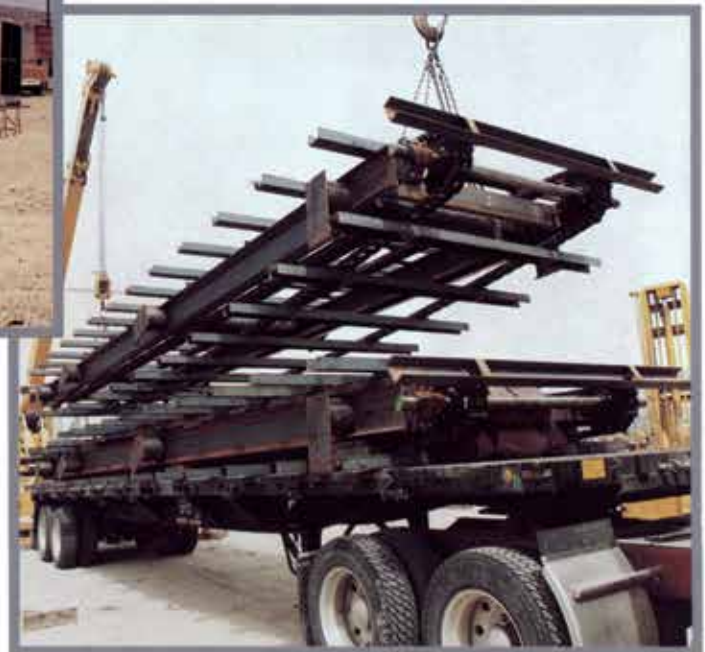
▶ Large drag conveyors for a pulp plant in Canada.
