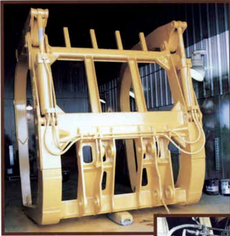
Repair and add reinforcing plates to a set of log forks. ▲
