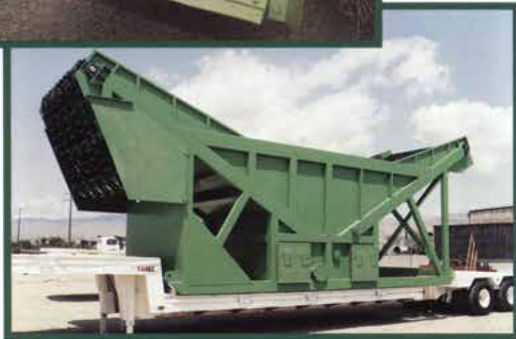
▲ Log yard flotation tank in a waste recovery system at an Eastern Oregon sawmill.
