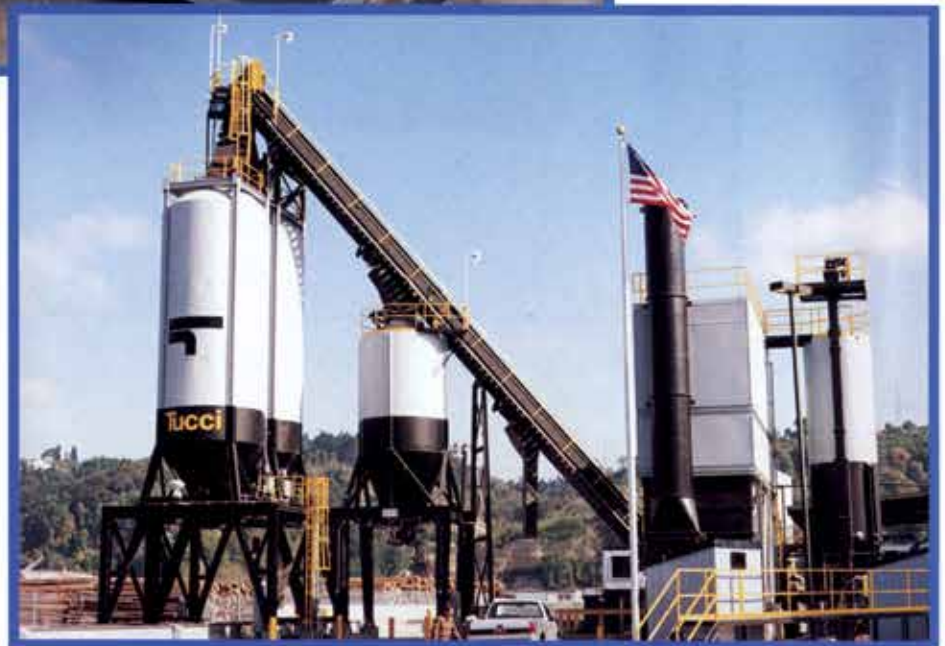
Two, 200 ton capacity silos and one, 36 in. x 88 ft. drag conveyor with splitter chute and two drop out gates in Tacoma, Washington. ▶
