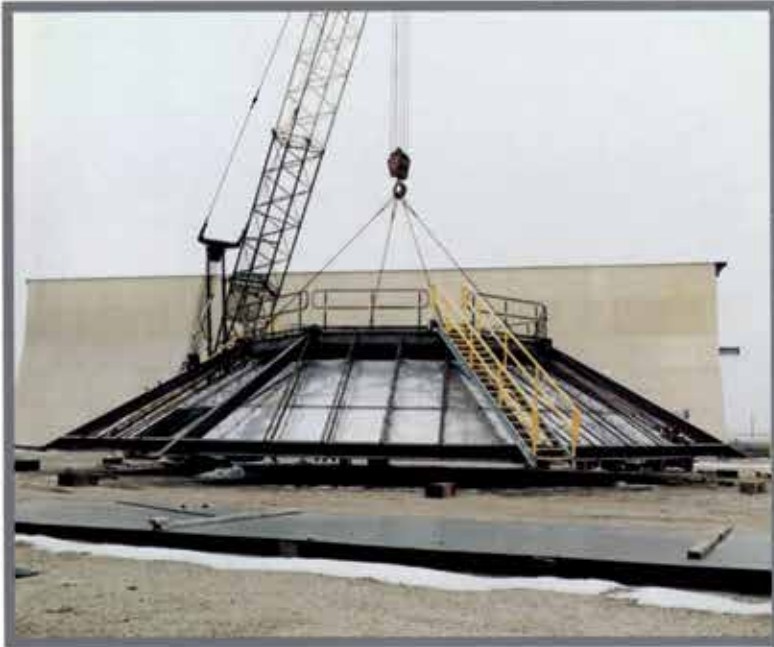
▲ One of two off-gas hoods fabricated and assembled for an environmental services company in Washington.
