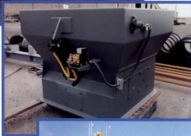
Standard 6,000 lb. asphalt batch hopper. ▶
