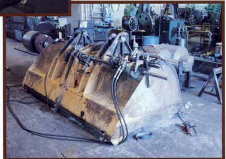
Bucket pivots being rebored and rebushed. ▲
