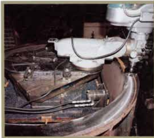
▶ Machining of a press roll shaft in a 80 in. x 30 ft. lathe.
